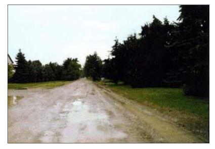
Applying a Double Chip Seal Surface will eliminate the need for grading and dust control. If your base is not sufficient, we will add base material and grade your existing road to ensure proper drainage. Ditches and drains that work are most important for making any new road surface work. The picture at left shows the road condition of Dinser Road in Novi before our preparation.
